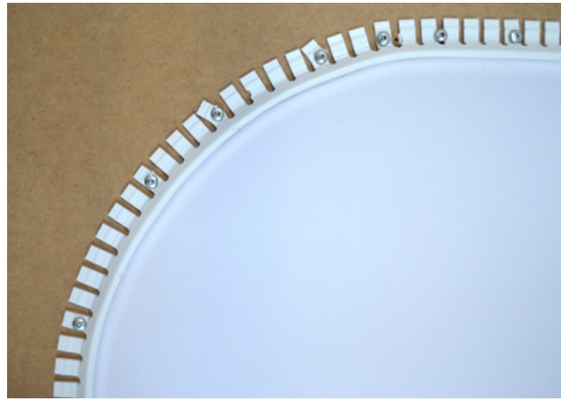
Image B15 - DESCOR ® APC-profile – minimum bending radius = 20 cm
